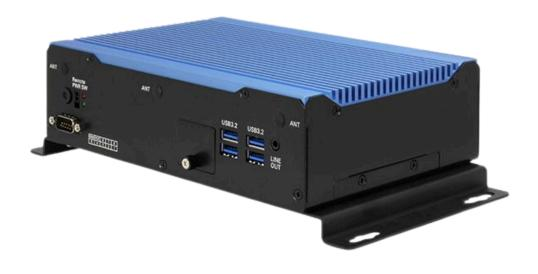
BOXER-6647-MTH is a Fanless Compact Embedded Computer with Intel® Core™ Ultra 7/5 Processors. Intel® Core™ Ultra 5/7 Processor.
